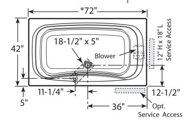
Product Shown: Signa® 6 Pure Air II Bath Right Hand Model: EA90 \* Measurements inside unit represent cutout in floor to allow for drain/overflow. Minimum Service Access dimensions given.
